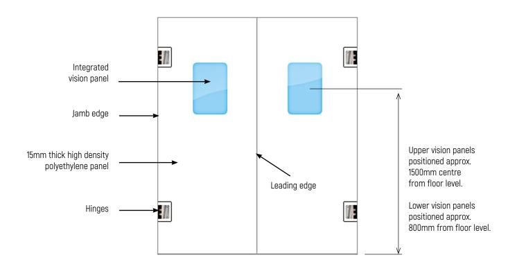
**Size:** Single – up to 1200mm x 2400mm (w x h). Pair – up to 2400mm x 2400mm (w x h).
