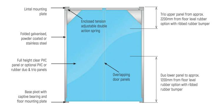
**Size:** Single – up to 1500mm x 3000mm (w x h). Pair – up to 3000mm x 3000mm (w x h).
